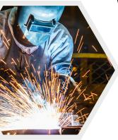
Workmanship is an essential aspect of both welding and brazing. Technical ability and skill are critical to achieving consistent welds with the appropriate mechanical properties. Thus welders are required to be qualified in undertaking welds to a particular WPS. This involves the production of a test piece which is then subject to testing. This is known as welder qualification.
